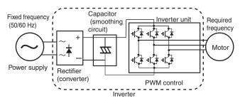
The voltage output from the inverter is in pulse form. The pulses are smoothed by the motor coil, and a sine wave current flows. As a result, the output from a general-purpose inverter cannot be used for equipment other than motors.
