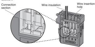
3. Insert a flat-blade screwdriver into the release hole and gently reset the lever. You should hear the operation lever reset.
