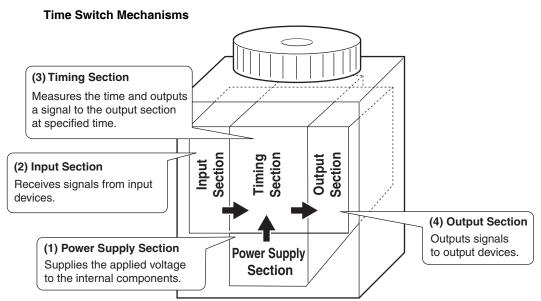
However, most models of Time Switches do not have an input section.
