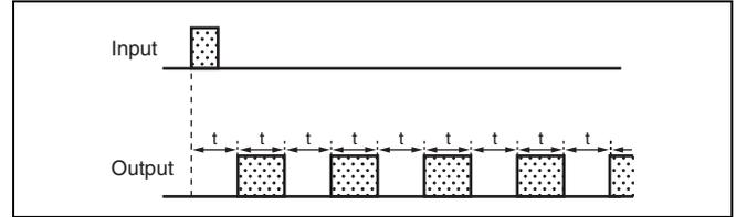
With flicker operation, an output repeatedly turns ON and OFF at the set time after an input is received.
