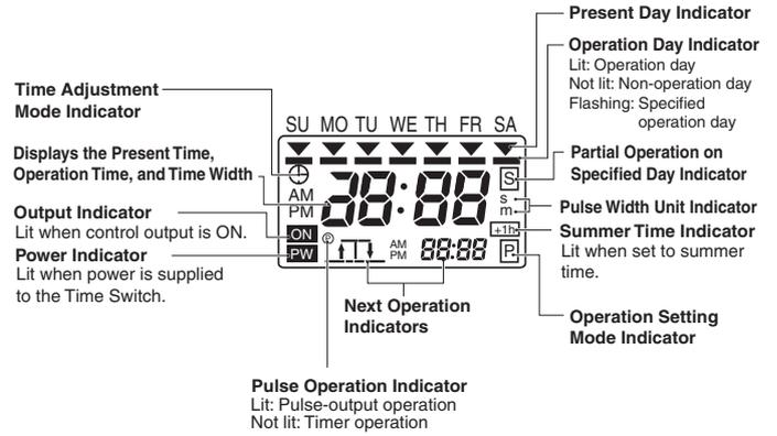
Run mode: Displays the direction (i.e., ON or OFF) and time of the next output operation.
