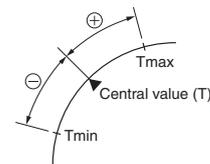
If the settings of an Analog Timer is changed while it is performing time-limit operation, the following operation will result.
