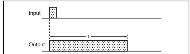
With interval operation, the output turns ON at the same time as the input and the output turns OFF after a set time.
