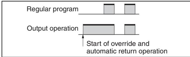
With override and automatic return operation, the output ON/OFF switch and the Write Key are used to hold the control output ON until the next OFF time.
