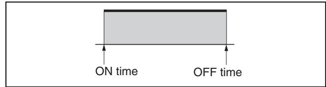
With timer operation, the Time Switch controls the output according to the set ON and OFF times.
