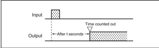
With ON-delay operation, the Timer receives an input and then an output signal is output by switching the Timer contacts after a set time delay.
