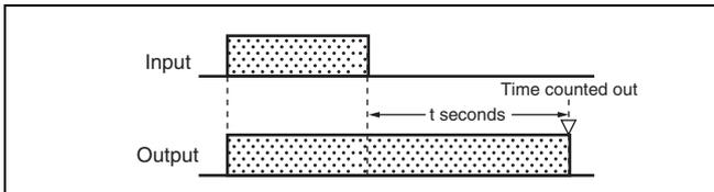
With OFF-delay operation, the output turns ON at the same time as the input and then the output turns OFF when the Timer contacts switch after the set time has expired. The set time is calculated from when the input turns OFF.
