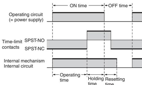
The resetting time of the Timer is the period of time during which all the internal components including the contacts, pointer, and the circuit components, such as the capacitor, of the Timer are reset.
