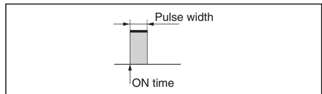
With pulse-output operation, the Time Switch outputs a pulse of a specified time width at the set ON time.
