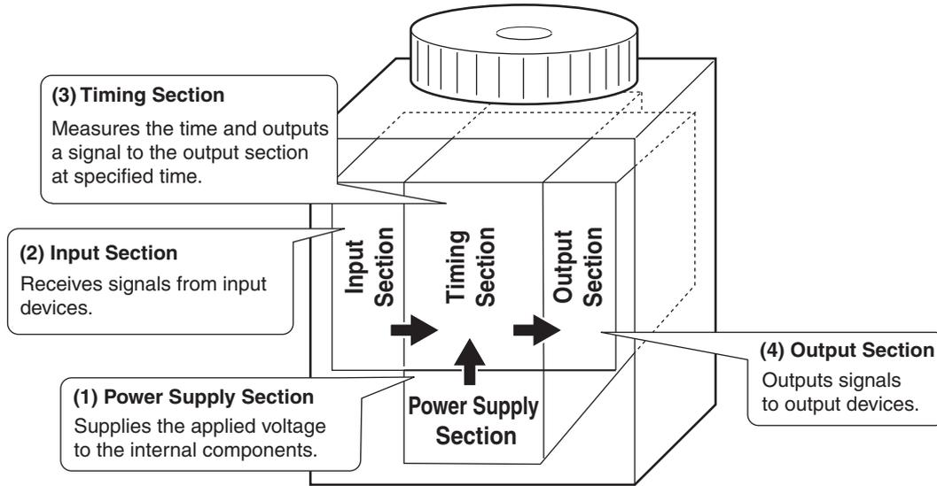
However, most models of Time Switches do not have an input section.
