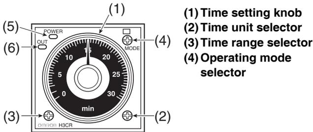
**Note** A variety of time ranges can be set with the H3CR-A using the time unit selector and time range selector.
