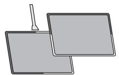
Transparent conductive layers are formed over the entire surface of the top and bottom layers. One of the two layers constructs the X-coordinate circuit while the other layer constructs the Y-coordinate circuit. The resistance ratio at a touched position is detected as an analog value.
