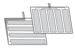
Transparent conductive layers strips formed on the top and bottom layers are at right angles to each other. When the panel is touched, the position is detected in the X and Y coordinates.
