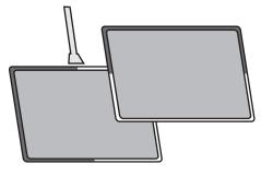
Transparent conductive layers are formed over the entire surface of the top and bottom layers. One of the two layers constructs the X-coordinate circuit while the other layer constructs the Y-coordinate circuit. The resistance ratio at a touched position is detected as an analog value.
