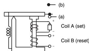
When current flows through coil A, the electromagnet (made of semi-hard material) is magnetized and the armature is attracted to the core.
