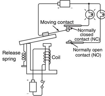
No current is applied to the operating coil, so the electromagnet does not operate. The armature is pulled by the force of the release spring in the counterclockwise direction and, as a result, the moving contact makes contact with the normally closed contact (turns ON) and the normally open contact stays disconnected from the moving contact (remains OFF).
