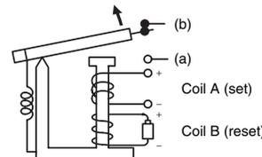
If a current is applied to coil B, which is wound in the opposite direction to coil A, the residual magnetic flux in the semi-hard magnetic material will reduce and the magnetic attraction will weaken. The power of the release spring will become stronger than the magnetic attraction, so the armature will release and the relay will be in a relaxed state.
