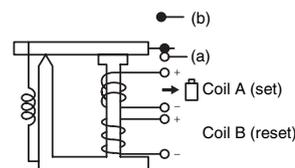
In the set state, the residual magnetic flux in the semi-hard magnetic material (material that has properties similar to a permanent magnet) will keep the armature attracted to the core even if a current is no longer applied to coil A.
