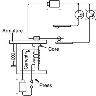
When current flows to the operating coil the electromagnet is magnetized and the armature is drawn to the core. As a result, the moving contact moves away from the normally closed (NC) contact and connects (turns ON) the normally open (NO) contact.
