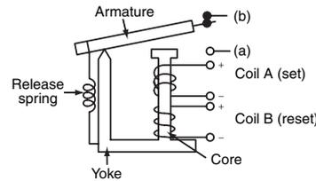
The diagram shows the relay in the relaxed state.
