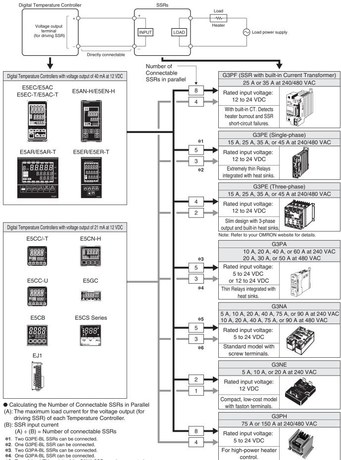
$<sup>\</sup>boldsymbol{*5.}$  Two of the -UTU models of the G3NA SSRs can be connected.
