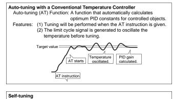
Self-tuning (ST) Function: A function that automatically calculates optimum PID constants for controlled objects. Features: (1) Whether to perform tuning or not is determined by the
