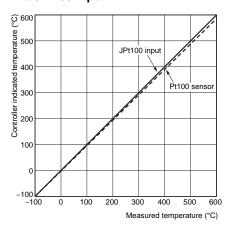
Indicated Temperature when Connecting JPt100 Sensor to Pt100 Input
