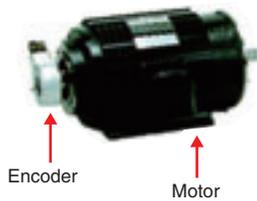
With this method, the inverter monitors the output voltage, the output current, and the encoder feedback from the motor. The encoder feedback is used to adjust the output waveform to perform precise speed control.
