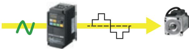
This type of control, in which the frequency and voltage are freely set, is called pulse width modulation, or PWM. The inverter first converts the input AC power to DC power and again creates AC power from the converted DC power using PWM control. The inverter outputs a pulsed voltage, and the pulses are smoothed by the motor coil so that a sine wave current flows to the motor to control the speed and torque of the motor.
