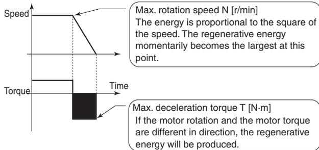
$$\text{Resistance of braking resistor: } R \leq \frac{V^2}{1.048 \times (T - 0.2 \times T_m) \times N \times 10^{-1}}$$
