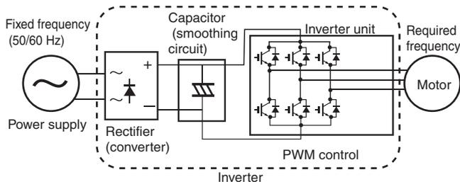
The voltage output from the inverter is in pulse form. The pulses are smoothed by the motor coil, and a sine wave current flows. As a result, the output from a general-purpose inverter cannot be used for equipment other than motors.
