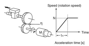
Speed (rotation speed) vs. Time graph showing acceleration time  $t_a$ .
