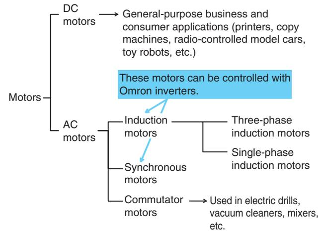
As induction motors can be used to achieve simple speed control at a relatively low cost, they are used in many applications. They can be operated just by connecting an AC power supply, so installation is extremely easy. Generally, a cooling fan is attached to the back to help dissipate heat generated by the motor.
