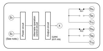
**Note:** The above diagram is for a rated voltage of 200 or 220 VAC. Power is supplied to S<sub>0</sub> and S<sub>1</sub> for 100 or 110 VAC.
