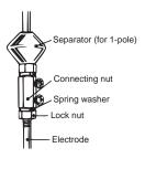
Note: 1. The spring washer comes with the lock nut. Contact your OMRON representative to purchase a replacement if the spring washer wears out or is lost.
