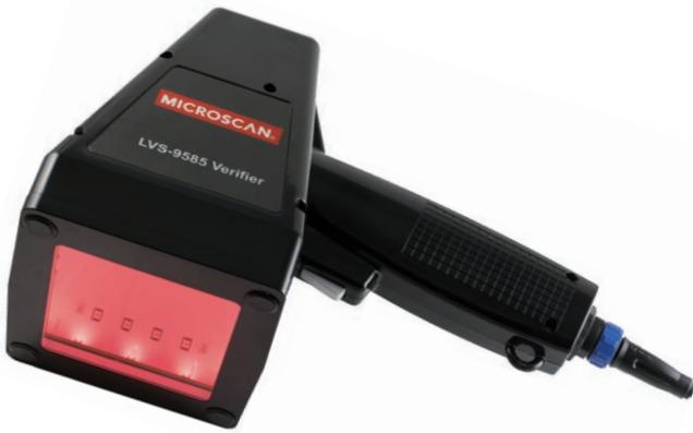
The LVS-9585 is a high-performance handheld solution for off-line barcode verification to ISO / IEC, ANSI, and GS1 standards. Featuring a high-resolution 5.0 megapixel camera, the LVS-9585 reads and analyzes linear (1D) and two-dimensional (2D) codes up to 76.19 mm wide and up to 57.15 mm tall. 1D and 2D direct part marks (DPM) of up to 44 mm x 44 mm can be verified to MIL-STD-130, ISO, and GS1 standards.
