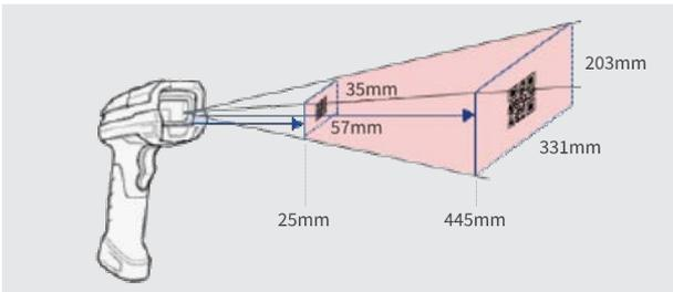
SR type provides easy alignment of a code reader with a code by its wide reading range and reading distance. Efficient manual code reading is possible.
