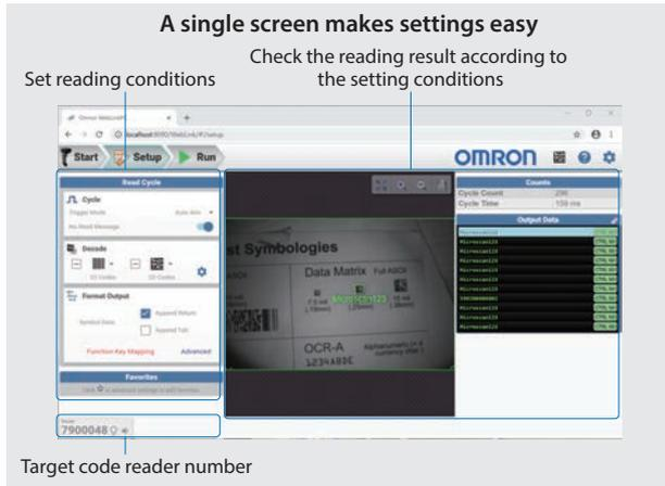
Easy setup with PC setup tool WebLinkPC. Setting most commonly used reading conditions and checking reading result are possible on a single screen, providing efficient setting.
