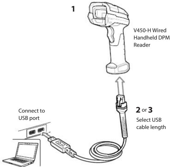
**Note:** This connection scheme is also used to connect the V450-H Handheld Code Reader to an Omron NA-Series Controller.
