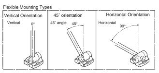
4. Using a shaft with an XY joint enables detection from above the production line.
