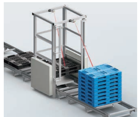
Detecting how many pallets are remaining
