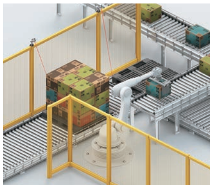
Sensing workpieces in a palletizing process
