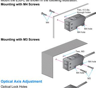
By inserting screws into the optical axis lock holes, the Mounting Bracket will be in the direction of the optical axis of the E3S-C.
