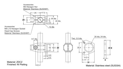
Note: Accessories 2-M3-L10 Cross Recessed Pan Head Screws (Attached to SW+JIS)
