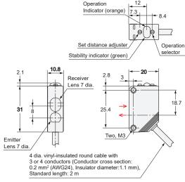
Note: Standard Model has four conductors and Laser Model has three conductors.
