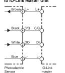
**Connector Pin Arrangement**
