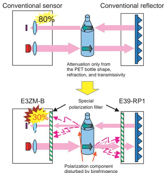
The excess gain of the E3ZM-B is doubled for both light-ON and dark-ON applications.
