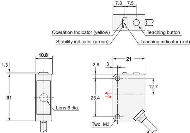
4 dia. vinyl-insulated round cable with 4 conductors (Conductor cross section: 0.2 mm<sup>2</sup> (AWG24), Insulator diameter: 1.1 mm), Standard length: 2 m
