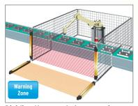
Dividing the zone between seriesconnected sensors
