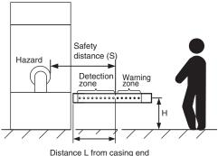
Distance L from casing end to detection zone
