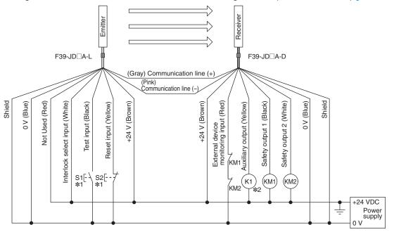
S1 : External test switch (connect to 24 V if a switch is not required)
