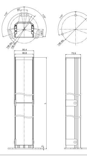
Material: Aluminum alloy (Housing) Hot rolled steel (Base) PBT resin (Cap) Glass mirror (Mirror)
