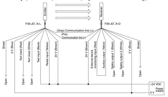
Minimum wiring required to check the operation of the F3SJ-B (Wiring for deactivated external device monitoring) (F3SJ-B CCC P25-02TS) [PNP Output]
