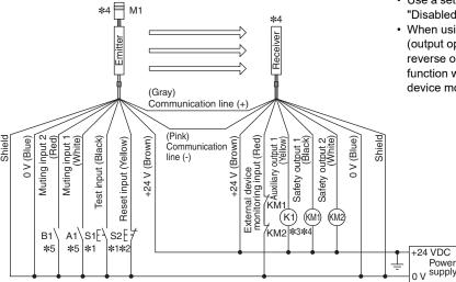
S1 : External test switch (connect to 24 V if a switch is not required)
