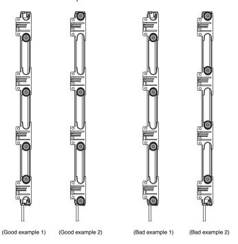
Mount One-touch M6 Brackets (or One-touch M8 Brackets) according to the mounting positions of the emitter and receiver. The positions of Intermediate Brackets mounted to the emitter and receiver must be aligned with each other.
