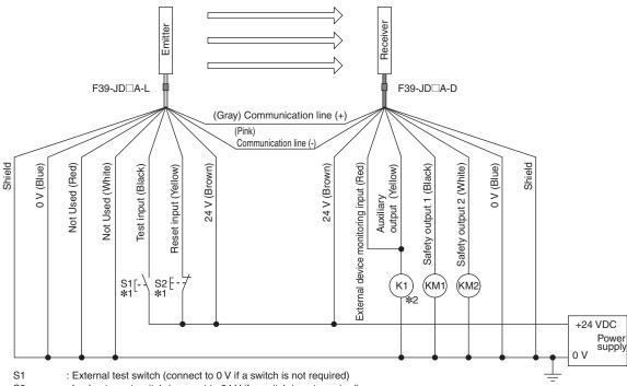
: Lockout reset switch (connect to 24 V if a switch is not required)
