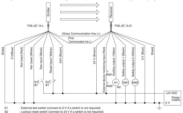
KM1, KM2 : Safety relay with force-guided contact (G7SA) or magnetic contactor
