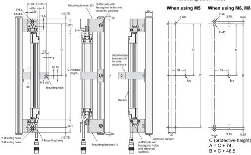
\*The four intermediate brackets (F39-PJ-MS) for side mounting are not provided.
