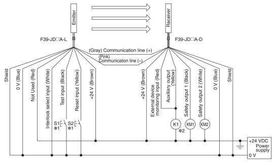
S1 S2 : External test switch (connect to 24 V if a switch is not required)
