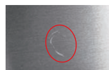
White scratch on shaded hairline finish
