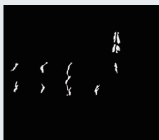
Overdetection of weld marks and shadows
