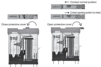
Keep the protective cover open when using the latching lever. Move until the latching lever clicks to the ON position (ON state). After use latching lever, in order to prevent malfunction, return the switch to contact normal position (OFF state), and make sure the protective cover is firmly closed.
