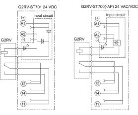
Equipped with a coil surge absorption circuit as standard.
