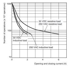
Switching capacity of DC resistive load
