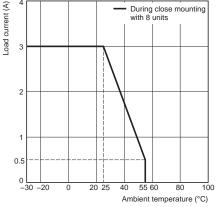
\*When eight or more are installed, install with 10 mm space between each. For details, please refer to Mounting on page 28.
