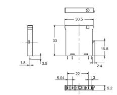
Terminal Arrangement/ Internal Connection Diagram (TOP VIEW) G3RV-D03SL(-H)
