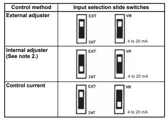
There is no slide switch combination with INT and 4 to 20 mA. Such combinations would have no current input control for 4 to 20 mA.
