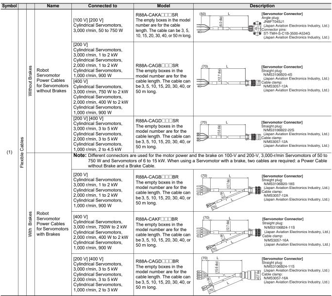
Note: Insert the cable length into the boxes in the model number of cables. (3 m: 003, 5 m: 005, 10 m: 010)
