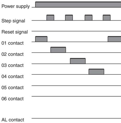
If an internal contact of the G9B is incorrectly turned OFF by the internal relay driving element that drives the internal contact due to external noise, the G9B will reset itself to its default status (i.e., contact 01 of the G9B will be turned ON) when the internal contact incorrectly turned OFF becomes active. In this example, contact 05 is incorrectly turned OFF.
