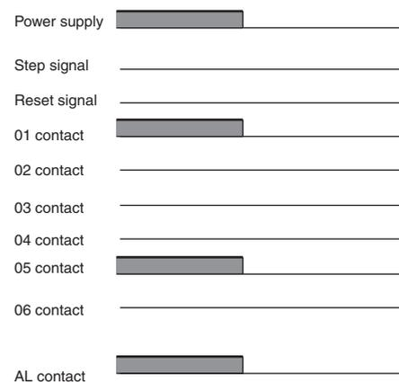
If an internal contact of the G9B is incorrectly turned ON by the internal relay driving element that drives the internal contact due to external noise, the G9B will reset itself to its default status (i.e., contact 01 of the G9B will be turned ON) and turn its alarm contact ON so that the ALARM indicator of the G9B will become lit. When the G9B is turned OFF, the alarm contact will turn OFF and the ALARM indicator will not be lit. In this example, contact 05 is incorrectly turned ON.
