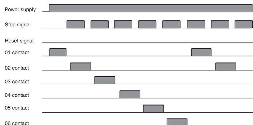
A different contact is selected in numerical order per step signal pulse. When the contact currently selected is 06, 01 will be selected with the next step signal input.
