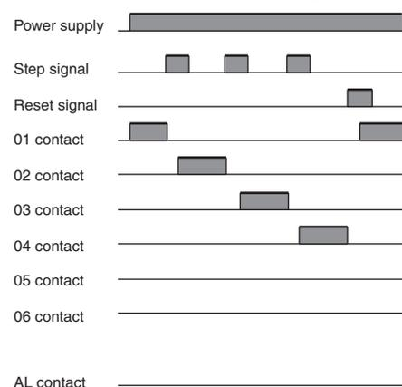
The G9B switches an active control terminal over to another control terminal and makes it active whenever the G9B receives a single step input pulse. If a reset signal is input to a control terminal of the G9B when the G9B is in stepping operation, terminal 1 of the G9B will become active.
