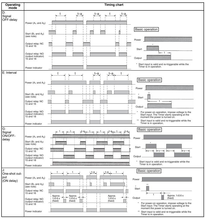
Note: The start input of the H3DS-ML□ model is activated by applying a voltage to B1 and A2 terminals. The voltage can be applied by turning on the contact between B1 and A1 (Refer to *Terminal Arrangement*).
