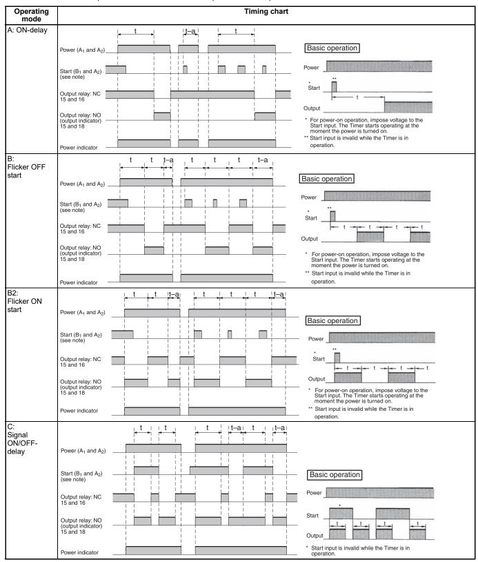
Note: The start input of the H3DS-ML□ model is activated by applying a voltage to B1 and A2 terminals.
