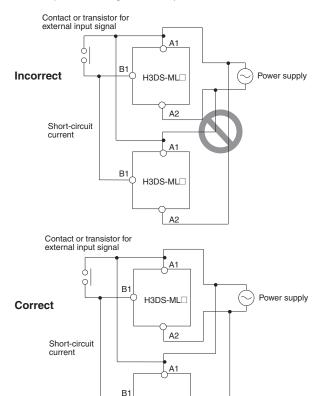
The H3DS Series is provided with a transformerless power supply system.
