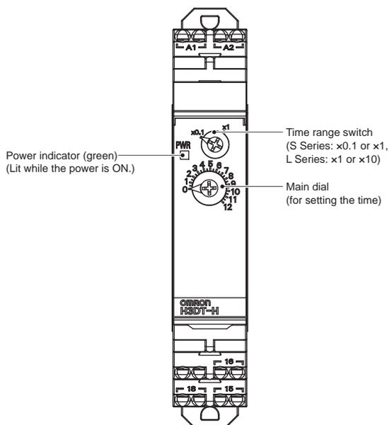
Note: If the switch is left between settings, proper operation may not be possible.
