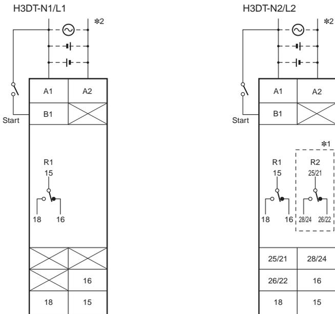
\*1. The relay R2 can be set to either instantaneous or time-limit contacts using the switch on the front of the Timer.
