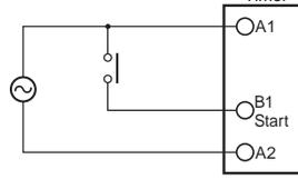
Operates when relay turns ON.
