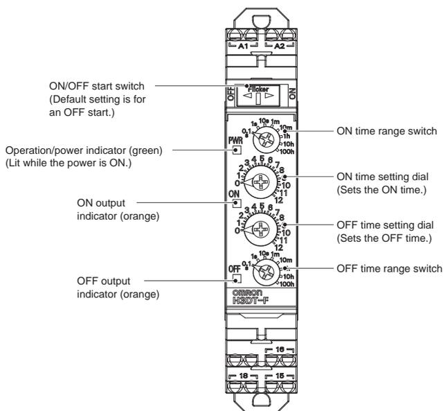
Note: If the switch is left between settings, proper operation may not be possible. Make sure that the switch is set properly.
