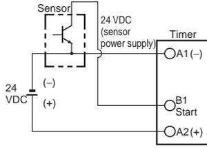
Operates when NPN transistor turns ON.
