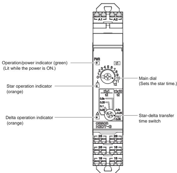
Note: If the switch is left between settings, proper operation may not be possible. Make sure that the switch is set properly.
