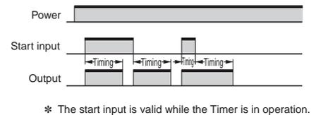
**Note:** 1. The reset time is 0.1 s min. Make sure the signal input time is 0.05 s or longer.
