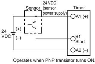
Operates when PNP transistor turns ON.
