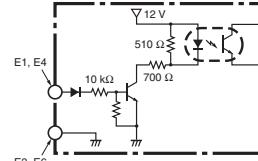
Note: A 2-wire DC sensor can also be connected. Check the ratings and characteristics tables, however, for the connection conditions.
