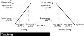
Settings for scaling can be made using the present measurement values instead of inputting values with the SHIFT and UP Keys. This is a convenient function for making the settings while monitoring the operating status.
