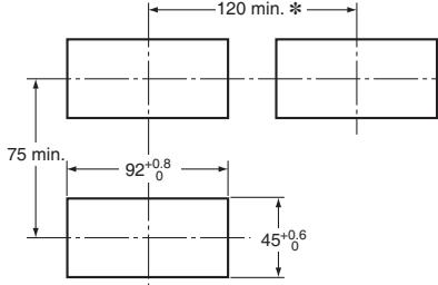
\*. Leave a distance of at least 140 mm when using the Watertight Cover Y92A-49N.
