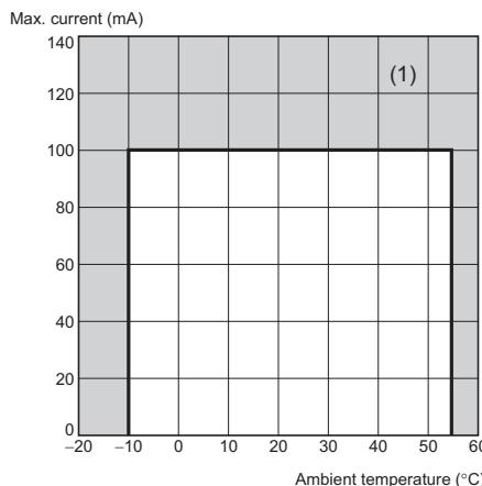
**Note:** 1. The above values are for standard mounting. The derating curve differs depending on the mounting conditions.
