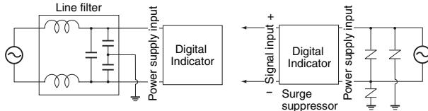
3. In order to prevent inductive noise, wire the lines connected to the terminal block separately from power lines carrying high voltages or currents. Do not wire in parallel with or in the same cable as power lines. Other measures for reducing noise include running lines along separate ducts and using shield lines.
