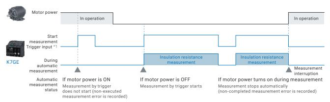
\*1. Refer to "Automatic measurement by arbitrary trigger input" on page 6 for details on trigger input.
