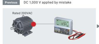
Voltage range must be selected in accordance with the rated value of the measurement target
