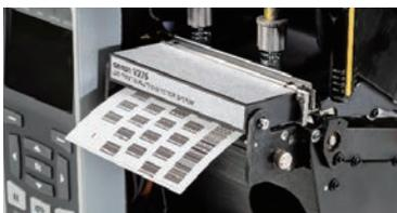
The barcode verification system integrated into a printer is also available.
