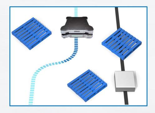
Unlike autonomous mobile robots (AMRs), automated guided vehicles (AGVs) require guides, which restricts their options for routing.
