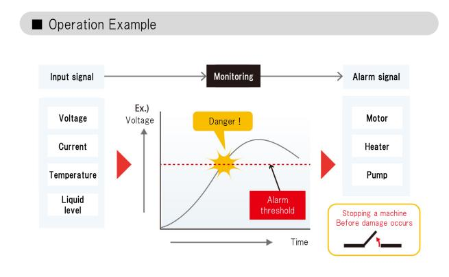
Input Signal voltage, current, temperature (from a thermocouple or platinum resistance thermometer), or liquid level (from an electrode) can be input.\*1
