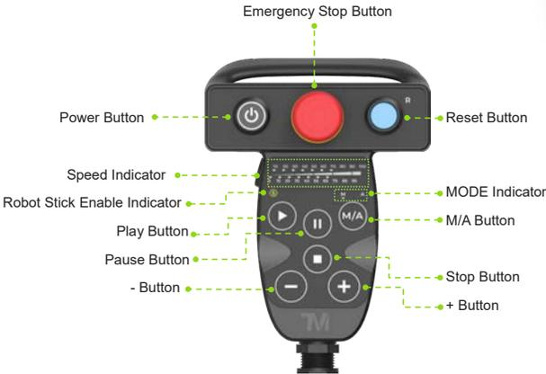
The new Robot Stick is designed to convert an **OMRON TM Screen** to a teaching pendant.
