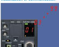
Visualization of the 7 communication modes provided on the front panels of amplifiers and controllers enables easy diagnosis without the need for host devices. In addition to making status confirmation easier for on-site operators, this also significantly reduces the time and labor required for installation, tuning, startup, and maintenance.
