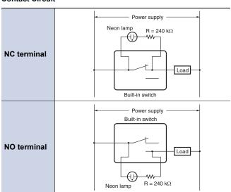
Note: If the wiring is as shown above, the operation of the respective parts will be as shown in the following table. The neon lamp is not wired when the Switch is delivered. Connect it as required.
