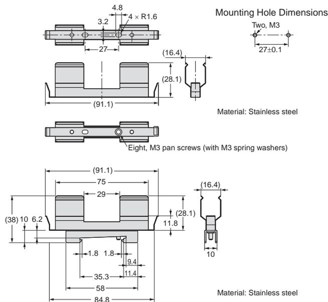
Sensor Head Mounting Bracket for Distance Compensation
