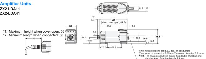
Standard length: 2 m, Minimum bending radius: 30 mm
