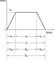
$$\text{Maximum Speed} \qquad v_0 = \frac{X_0}{t_0 - t_{\text{A}}}$$
