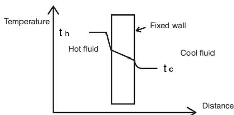
When this formula is applicable to the heat conductivity of the control panel under the following conditions, the heat conductivity Q will be obtained as shown below.
