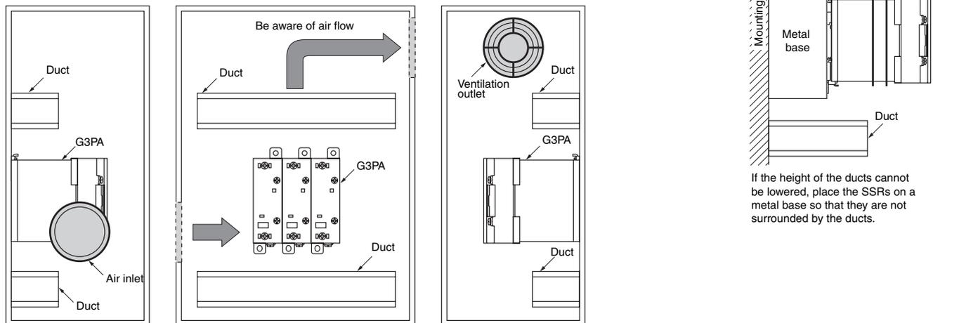
If the air inlet or air outlet has a filter, clean the filter regularly to prevent it from clogging and ensure an efficient flow of air.
