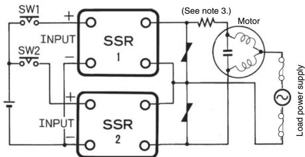
**Note: 1.** The voltage between the load terminals of either SSR 1 or SSR 2 turned OFF is approximately twice as high as the supply voltage due to LC coupling. Be sure to apply an SSR model with a rated output voltage of at least twice the supply voltage.
