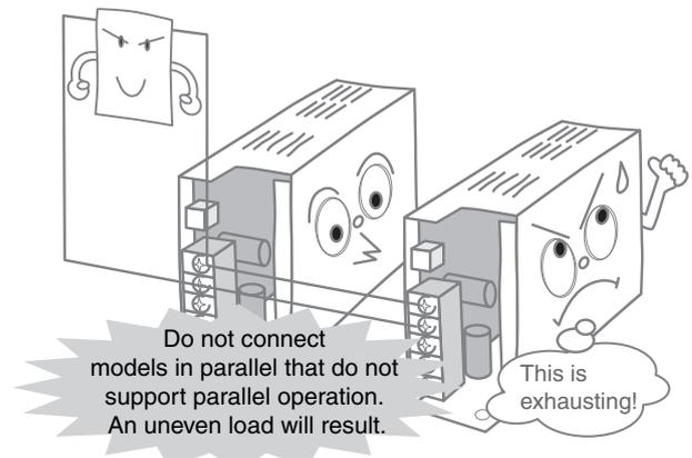
\* For details, refer to *Series, parallel, and  $\pm$  output operation* in the *Check point* column of the table on page 13.
