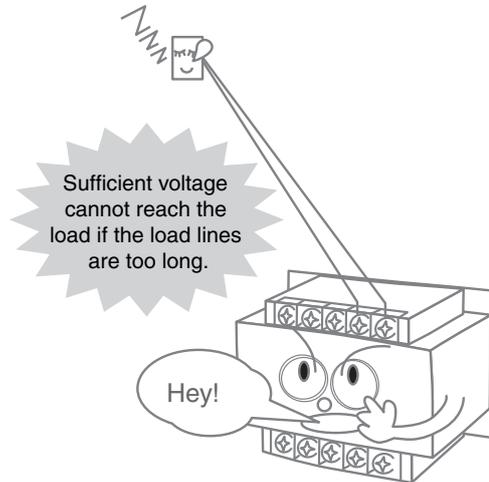
\* For details, refer to *The voltage applied to the load is low.* in the *Problem* column of the table on page 17.
