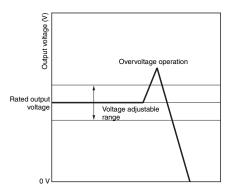
(When the overvoltage protection circuit operates, the Power Supply itself may be malfunctioning. When restarting the input power after the overvoltage protection circuit has operated, turn the input power ON with the load line disconnected and check the output voltage.)
