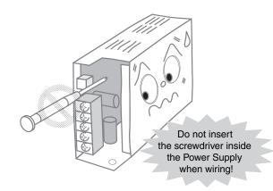
\* For details, refer to Terminal wiring in the Check point column of the table on page 13.
