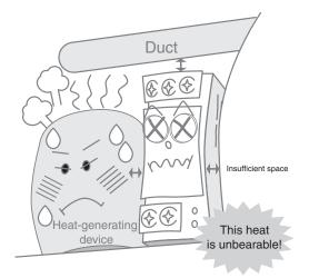
\* For details, refer to Installation location in the Check point column of the table on page 13.
