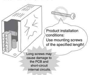
\* For details, refer to Installation conditions in the Check point column of the table on page 13.
