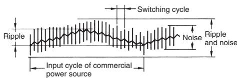
Since ripple and noise contain high-frequency components, the ground line of the oscilloscope must be shortened when making measurements. If the ground line is too long, it acts as an antenna which is influenced by radian waves and, consequently, the correct values of ripple and noise cannot be measured.
