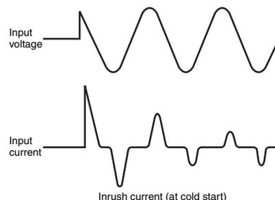
When two or more Switch-mode Power Supplies are used, the inrush current is the sum of the inrush currents for each Power Supply. Check the fusing characteristics of fuses and the operating characteristics of breakers, and select fuses and breakers so that external fuses will not burn out and breakers will not be activated by the inrush current.
