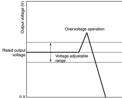
(When the overvoltage protection circuit operates, the Power Supply itself may be malfunctioning. When restarting the input power after the overvoltage protection circuit has operated, turn the input power ON with the load line disconnected and check the output voltage.)
