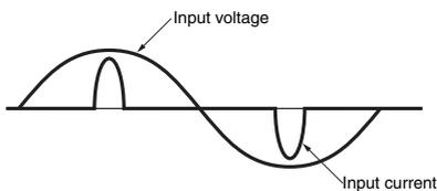
The power factor for devices that contain a lot of harmonic currents is low. The apparent power (VA) is larger than the actually consumed power (W), which increases the current. If there are too many of this type of device connected, Power Supply facilities with more leeway are required.
