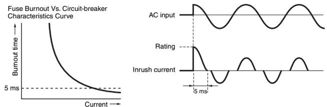
**Note:** The duration of the inrush current is 5 ms max. Therefore, the fusing characteristics require the inrush current to flow sufficiently for up to 5 ms.
