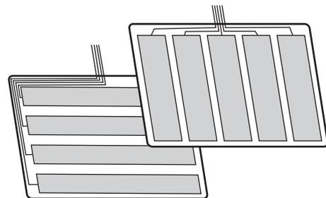
Transparent conductive layers strips formed on the top and bottom layers are at right angles to each other. When the panel is touched, the position is detected in the X and Y coordinates.
