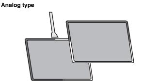
Transparent conductive layers are formed over the entire surface of the top and bottom layers. One of the two layers constructs the X-coordinate circuit while the other layer constructs the Y-coordinate circuit. The resistance ratio at a touched position is detected as an analog value. Matrix type
