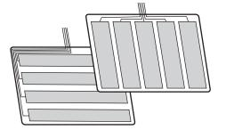
Transparent conductive layers strips formed on the top and bottom layers are at right angles to each other. When the panel is touched, the position is detected in the X and Y coordinates.
