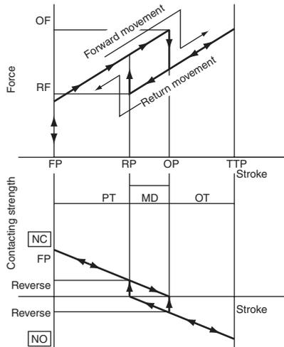
Force vs. Stroke vs. Contacting Force
