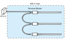
Note: 1. When wiring, be sure not to exceed the maximum possible wiring distances for both the connecting cable and the Sensing Band. Exceeding these distances may lead to faulty operation. Connect one Sensing Band to each Terminal Block.
