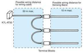
Note: 1. When wiring, be sure not to exceed the maximum possible wiring distances for both the connecting cable and the Sensing Band. Exceeding these distances may lead to faulty operation. Connect one Sensing Band to each Terminal Block.
