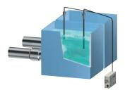
**Note:** Be sure to ground the baths if two or more K7L Sensors are used in the same tank in an explosion-prevention area.
