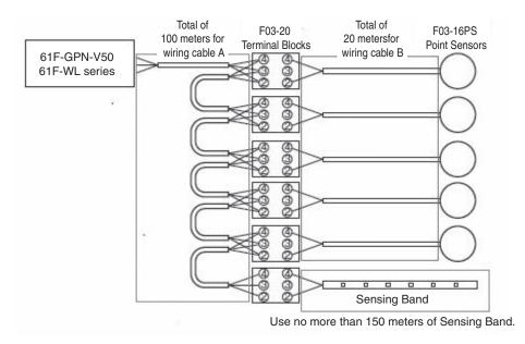
**<sup>\*2.</sup>** Point Sensors come with two 2-meter cables. Think of these cables as the wiring cables.
