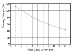
\* The 100% value is for a fiber cable with a length of 2 m (same for Through-beam and Reflective Models).
